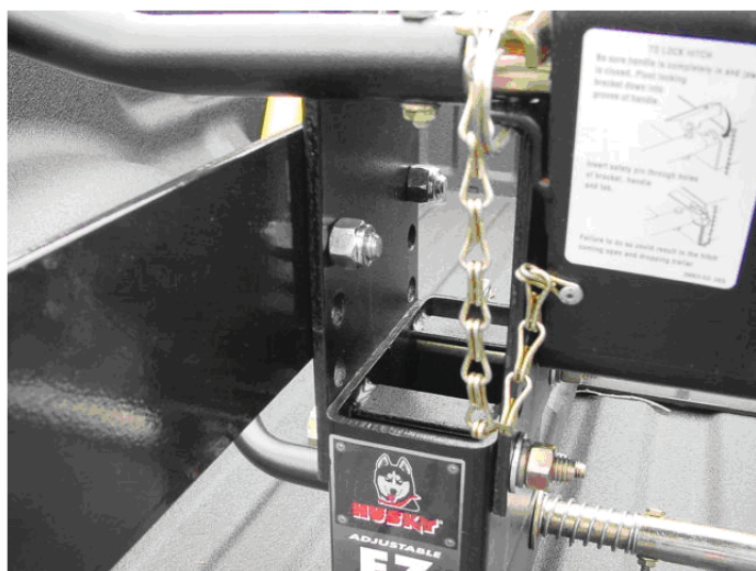
Figure 2- Side Plate Installed
