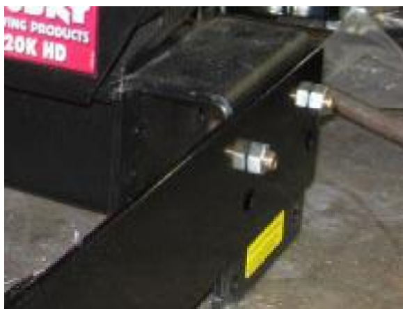
Figure 3-Left Side Plate attached
