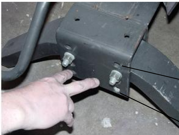
Figure 1-Determining Side Frame mounting bolts location
