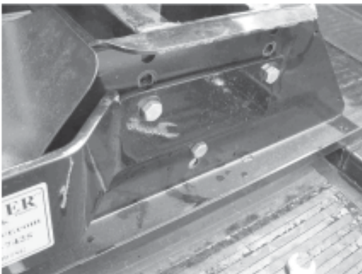
Figure 3-Right Side Plate Installation
