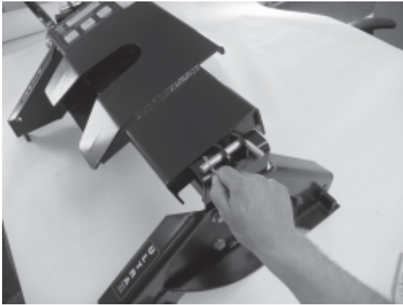
Figure 1-Removing Hitch Head Clip
