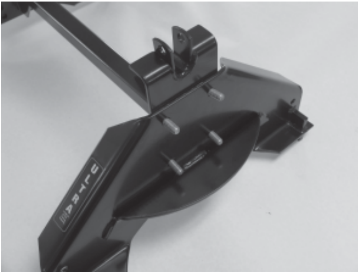
Figure 3-Right Side Plate installation
