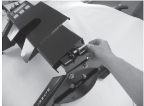
Figure 2-Removing Hitch Head Pin
